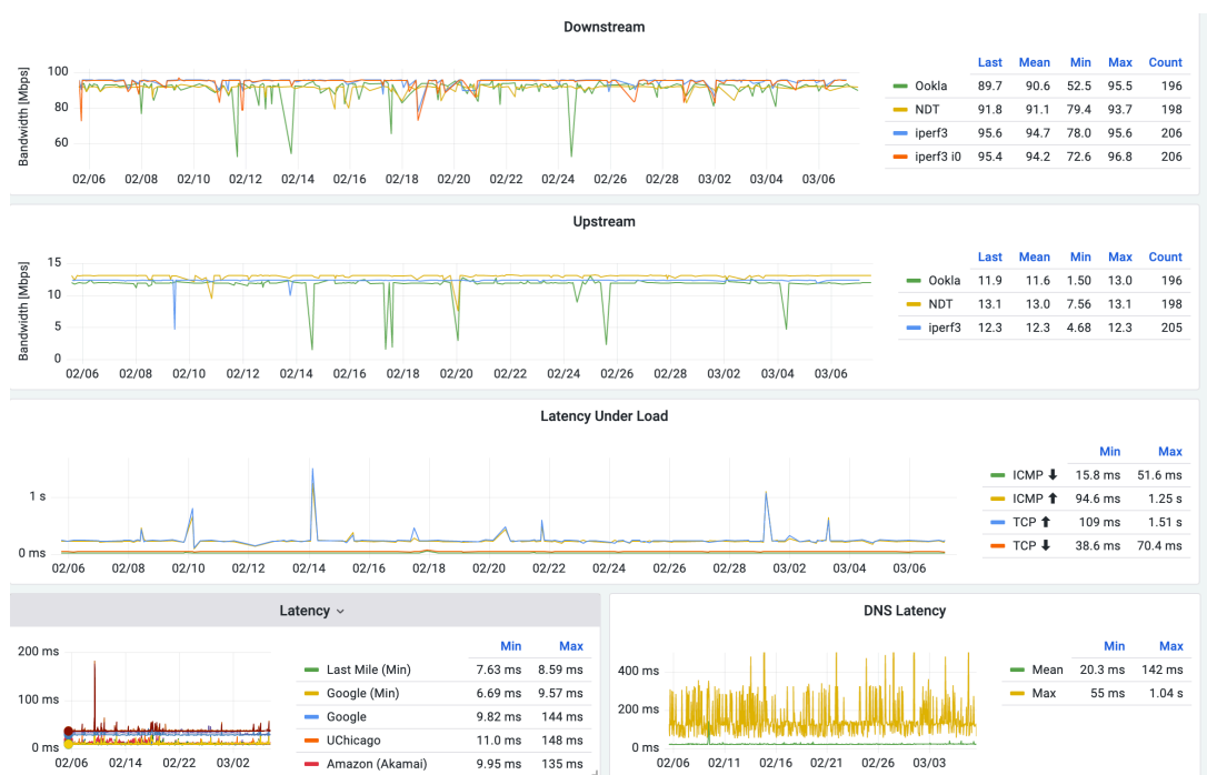
Figure 3: Real-time Netrics dashboard, showing a subset of the Internet performance metrics that are continuously collected from each participant.
